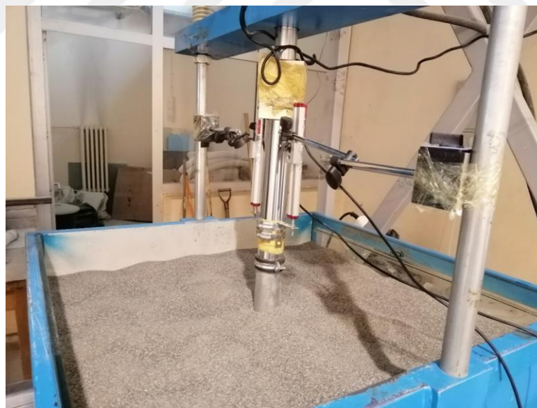
Figure 3.17 Two LVDTs installed in the model of experiment
