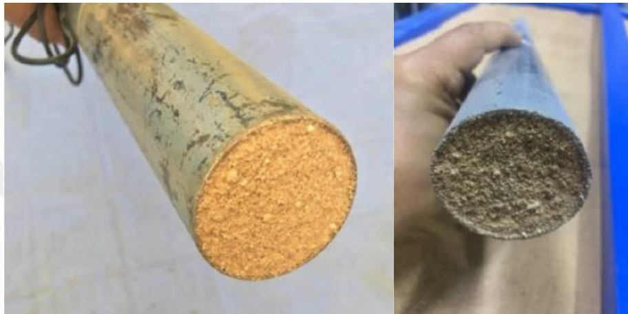
Figure 1.10 The flat shape of failure of below piles
