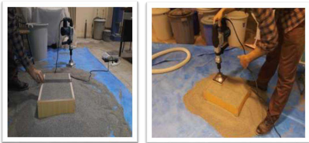
Figure 3.11 Calibration of the relative density of sand.
