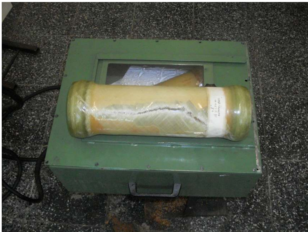
Figure 7.8 Fiber breakage damage mechanism
