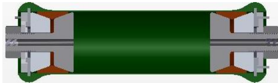
Figure 6.3 Closed-end internal pressure test apparatus.
