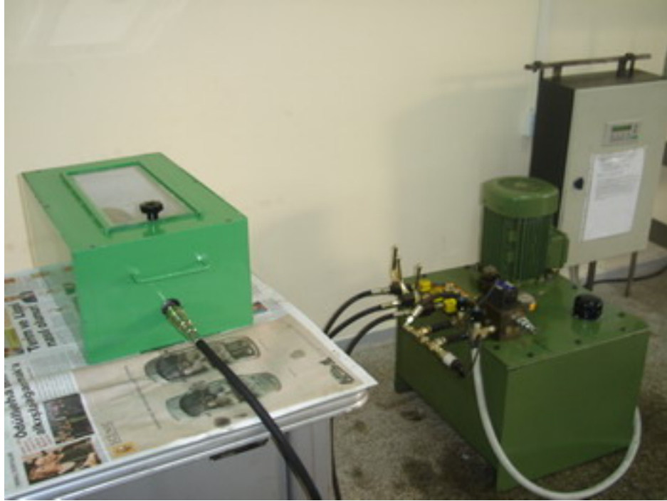
Figure 6.6 A PLC controlled servo-hydraulic testing machine.
