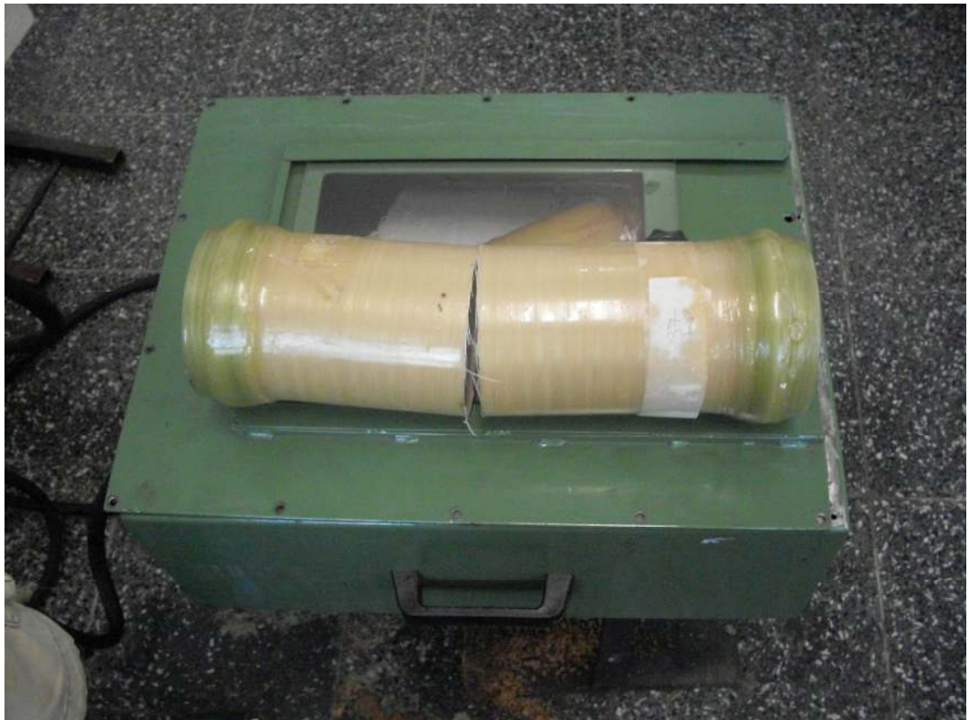
Figure 7.7 Fiber breakage damage mechanism
