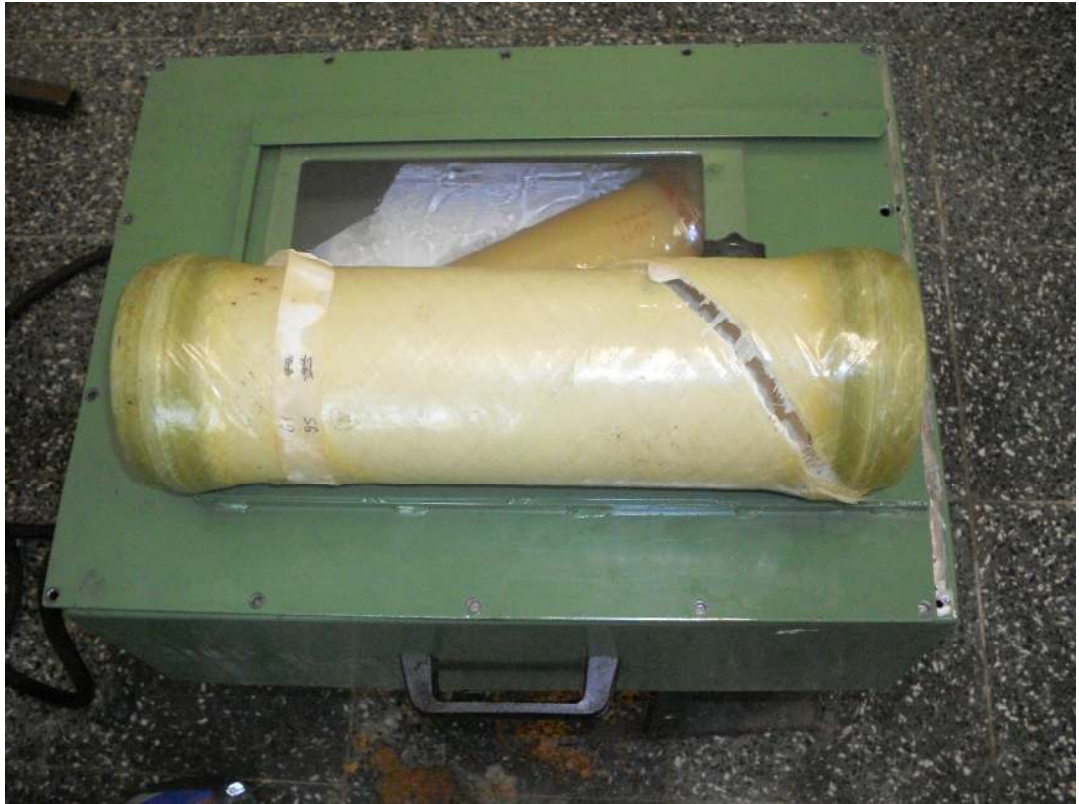
Figure 7.6 Fiber breakage damage mechanism
