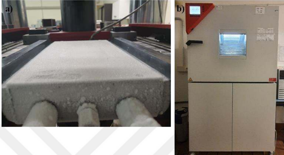
Figure 6.1. Small-scale test setup of Politecnico di Milano a) Temperature controlled steel plate, b) Climatic chamber
