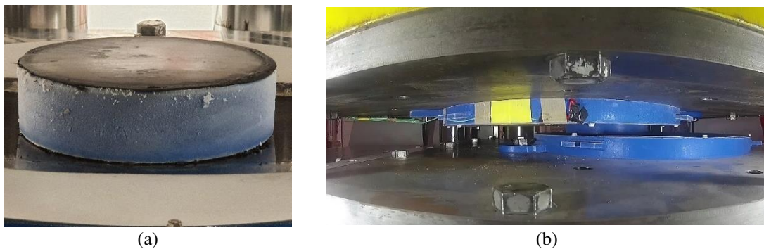
Figure 4.6. (a) The physical condition of both the slider and the stainless-steel plate, (b) a scene of the tested DCSS taken during the cyclic motion
