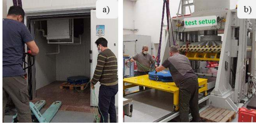
Figure 4.4. (a) The removal of the DCSS from the environmental chamber, (b) mounting of the DCSS to the test set-up
