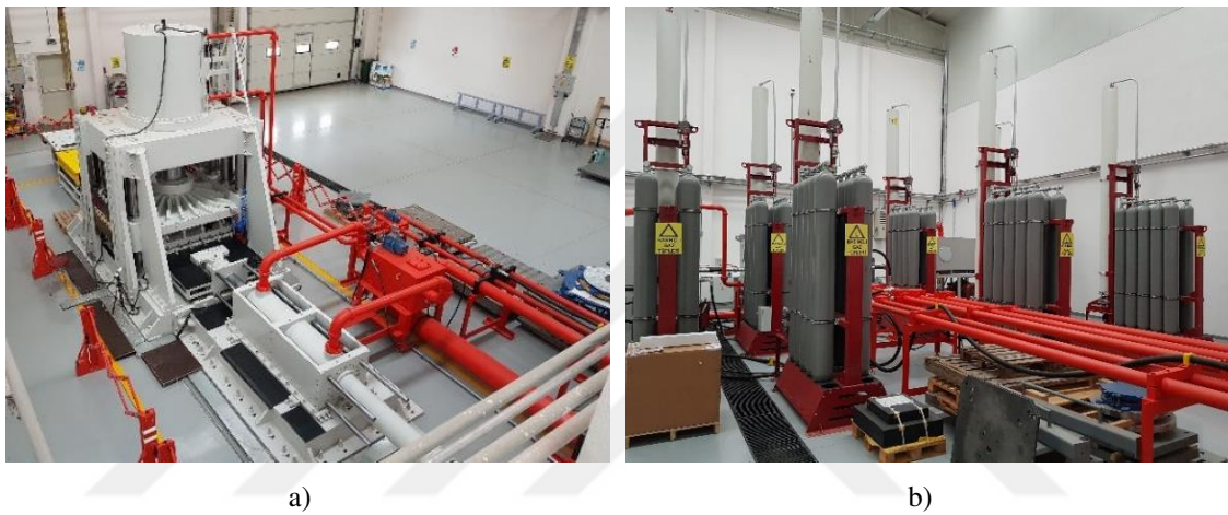
Figure 2.6. Seismic isolator test set-up (a), and accumulator sets used in Seismic Isolator Test Laboratory of Eskişehir Technical University (b).
