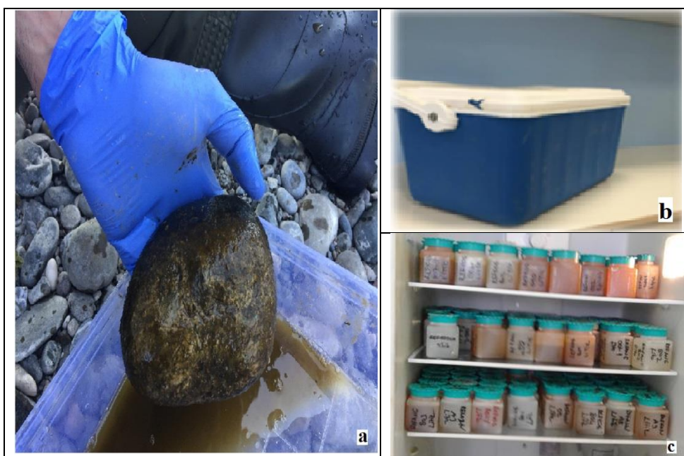
Figure 4.3 a) sampling; d) transfer in cooler with ice packs; and c) conservation in the laboratory of epilithic diatoms
