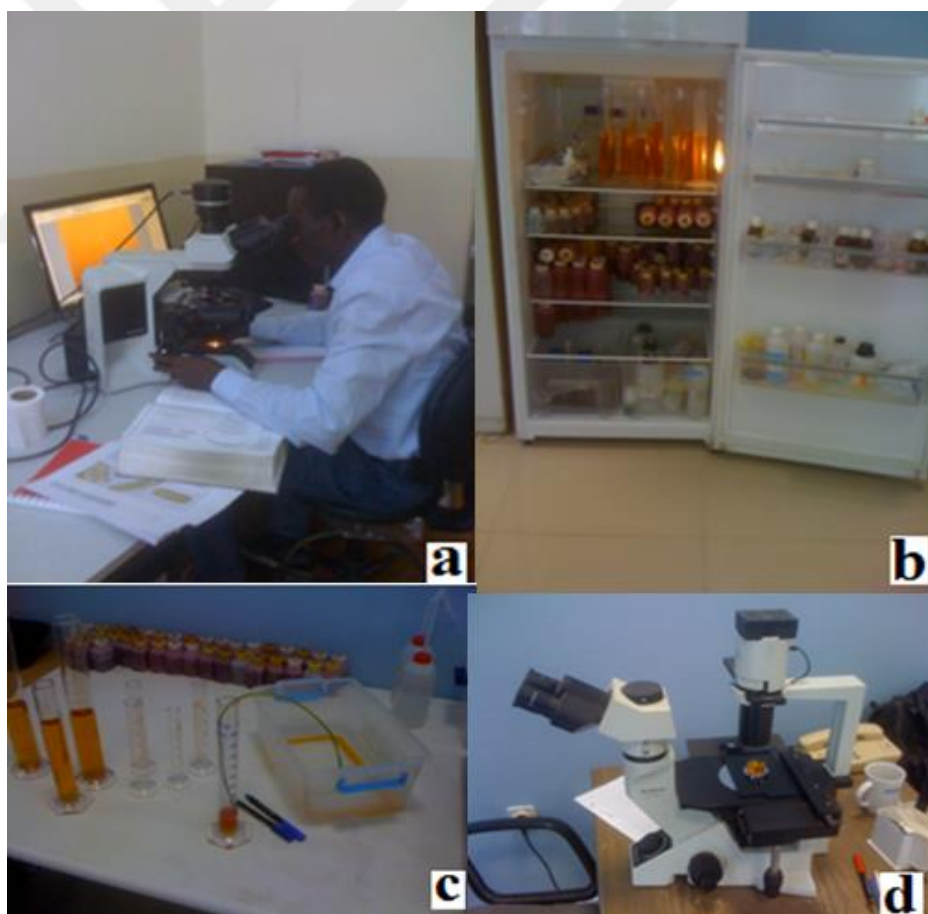
Figure 6.5 Phytoplankton identification and enumeration: a) identification, b) settling (24-48 hours), c) siphoning process, and d) counting chamber on inverted microscope
