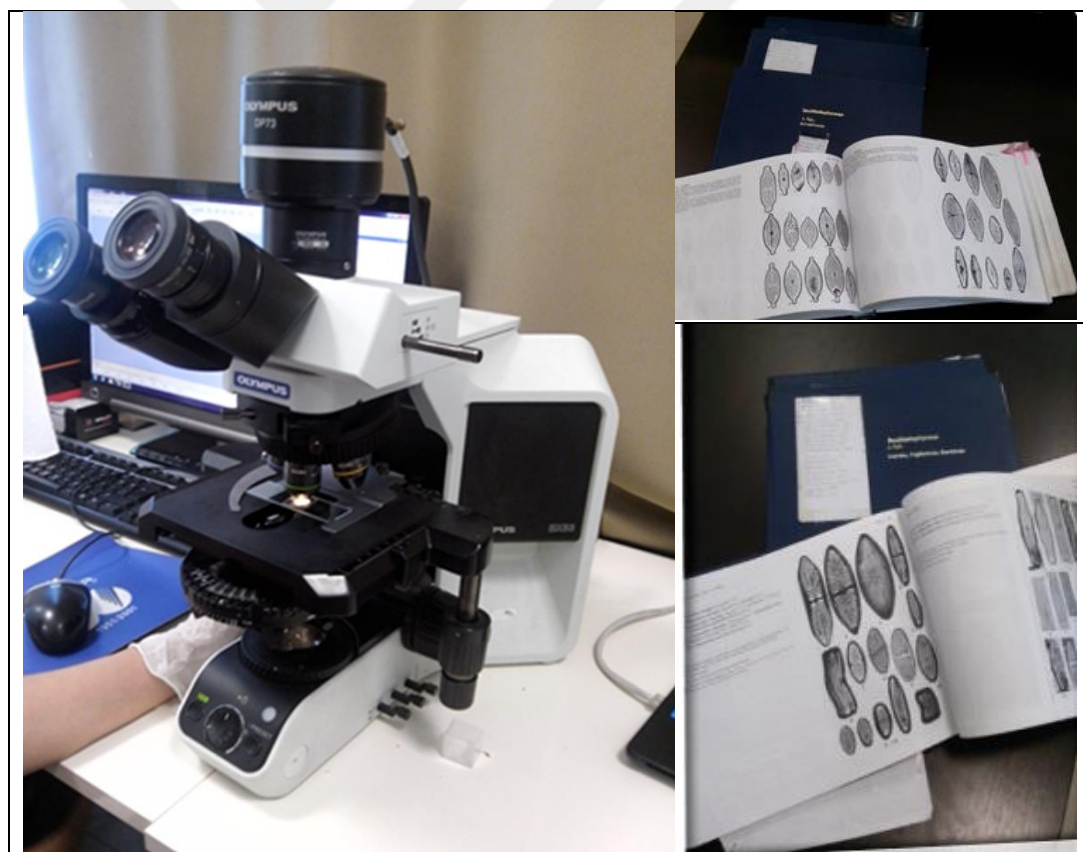
Figure 4.6 Diatom examination and identification under Olympus light microscope (Olympus BX53)
