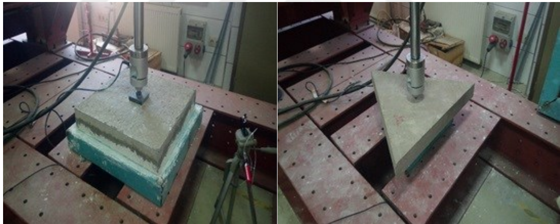
Figure 3.10. The two type of test Square panel & Triangular panel test
