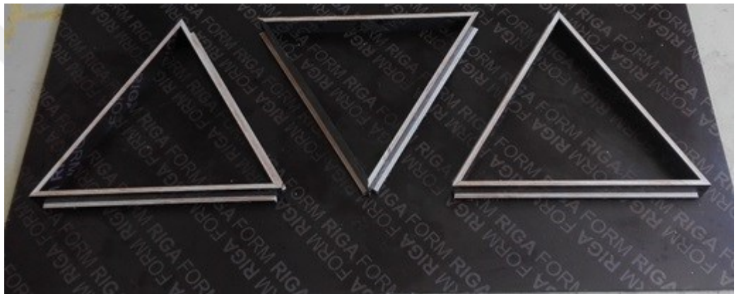
Figure 3.3. Triangular panels mold -800 mm.
