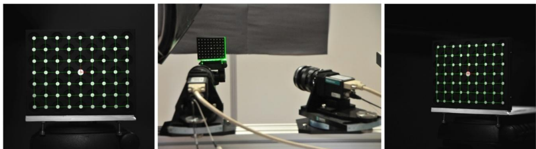
Figure 3.3 Position of the target with respect to cameras and images captured by the cameras for calibration
