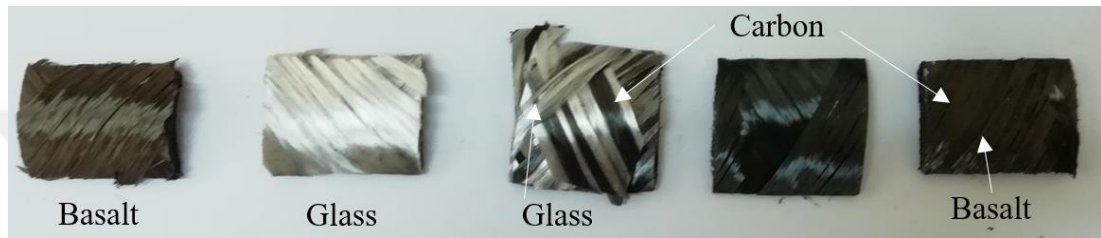
Figure 4.1 The samples after ignition loss tests
