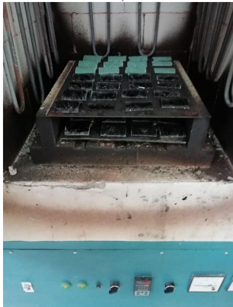
Figure 3.11 a) Samples, b) ignition loss test
