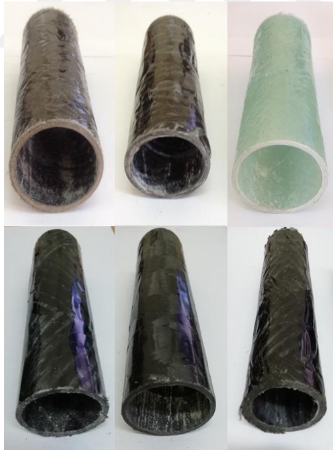
Figure 3.16 Samples for quasi-static radial compression test
