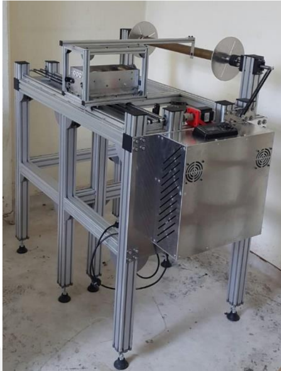
Figure 3.8 Final photograph of the filament winding machine
