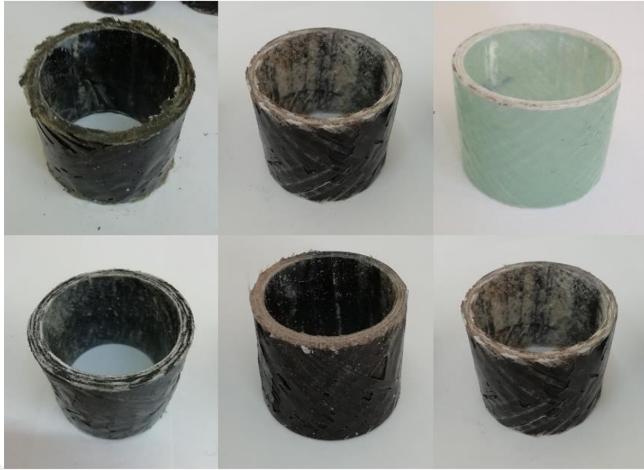
Figure 3.14 Samples for quasi-static axial compression test
