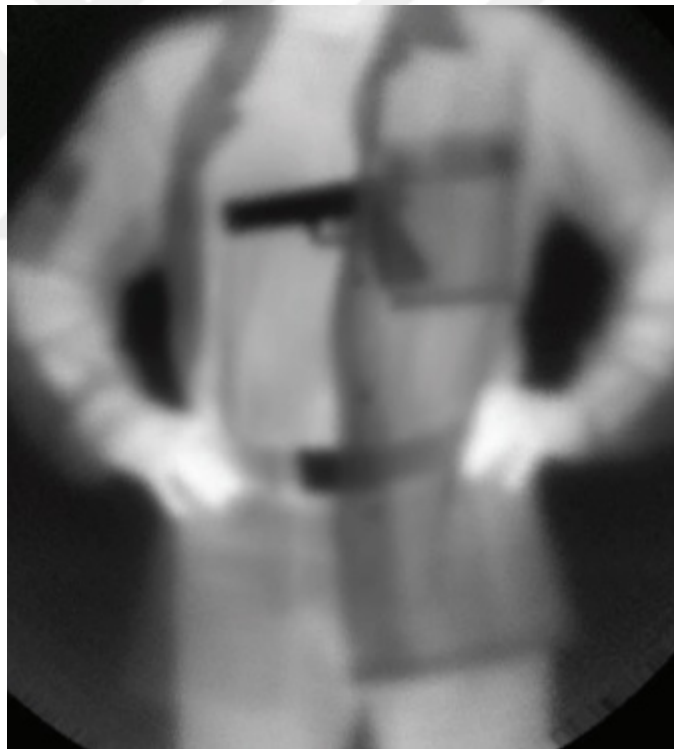
Figure 1.3: A (0.85-THz) image by THz camera depict the ability of showing the objects through clothes or fabric
