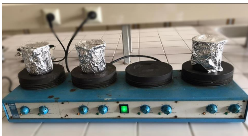
Figure 2.5. Stirring the samples with a magnetic stirrer.
