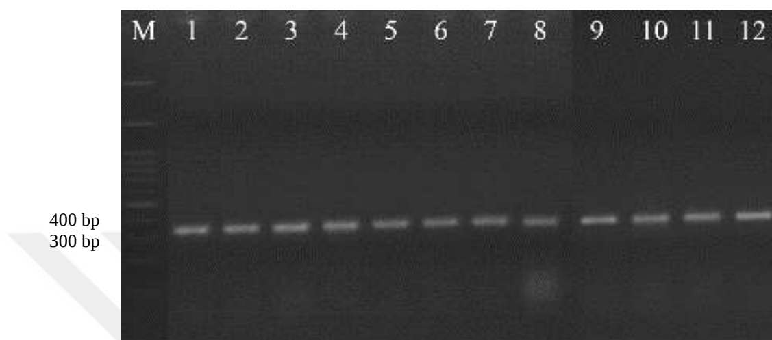
Figure 4.4 Amplicons obtained using species-specific primer pair MpKFI-MpKRI.
