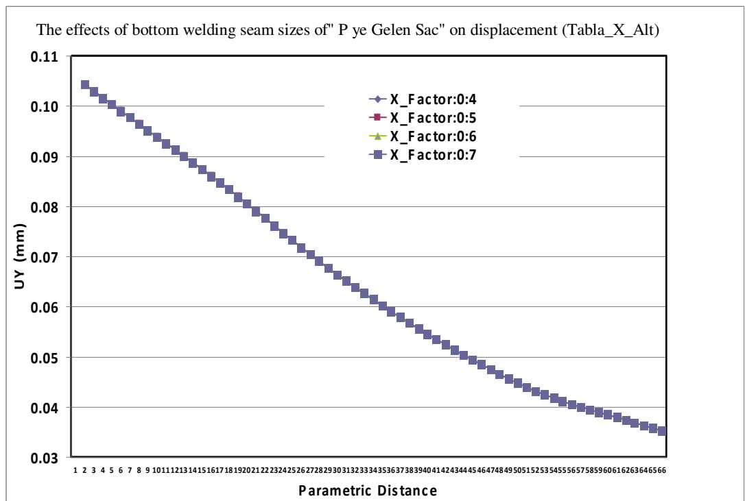
Figure 4.64 The effects of welding seam sizes on displacement
