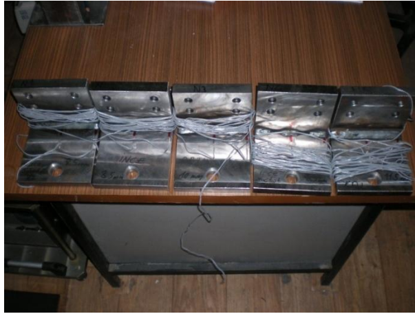
Figure 3.4 Welded L shaped test samples
