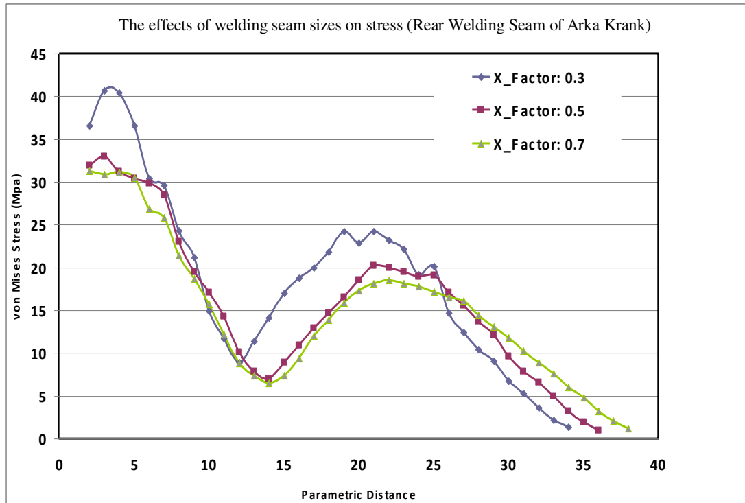
Figure 4.53 The effects of welding seam sizes on stress
