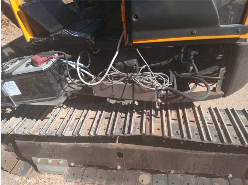
Figure 4.16. Test Equipment Installation of Compact Excavator Fuel Consumption Test
