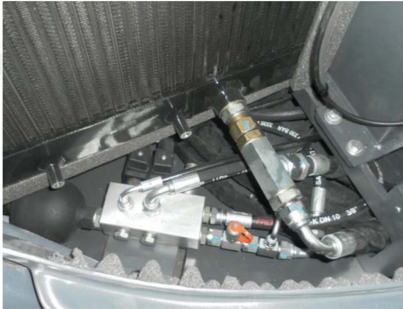
Figure 4.15. Check Points of Test Compact Excavator Hydraulic System Pilot Pressure Line (Mst User Maintenance Guide,2016)
