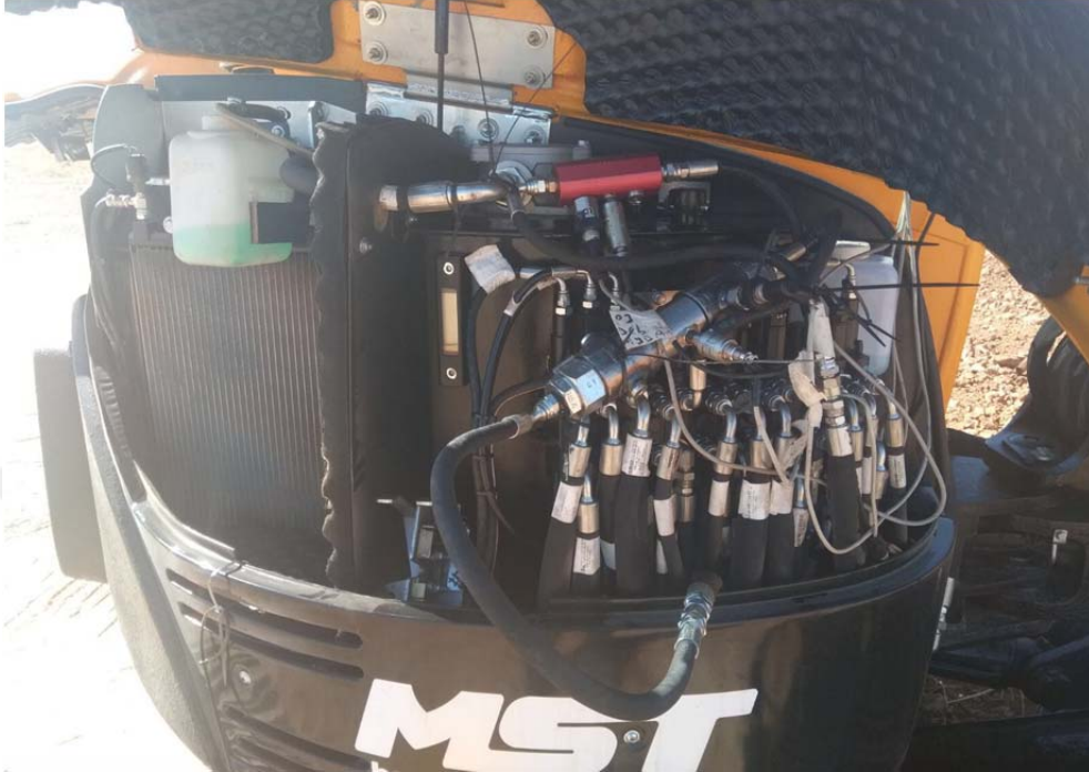
Figure 4.17. Test Equipment Installation for Compact Excavator Fuel Consumption Test
