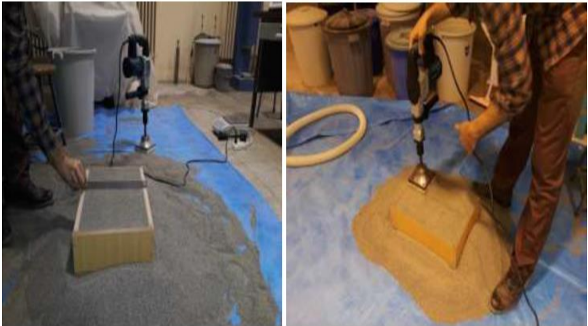
Figure 3.7. Calibration of relative density in the laboratory
