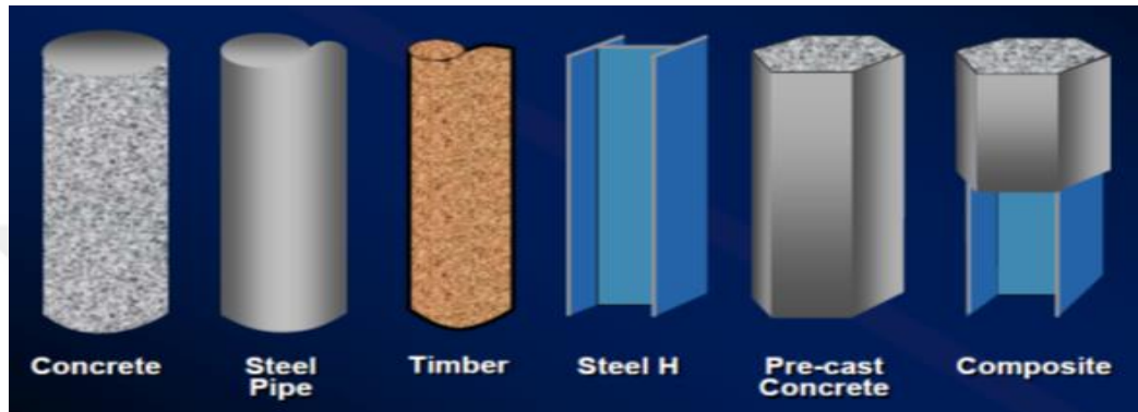
Figure 1.3. Types of piles based on shape and composition
