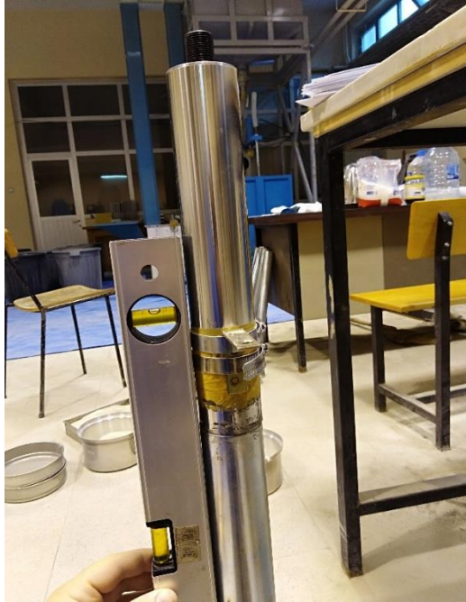
Figure 3.12. Attaching piles to the loading shaft
