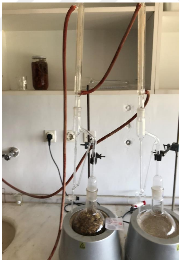
Figure 2.3: Clevenger apparatus for hydrodistillation.
