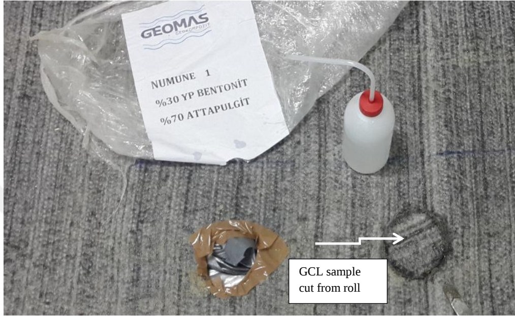
Figure 2.7 GCL sample cut from the GCL roll (Personal archive, 2015)
