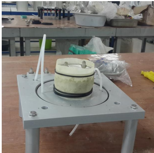
Figure 4 Fitting latex membrane and sliding O-rings (Personal archive, 2015)
