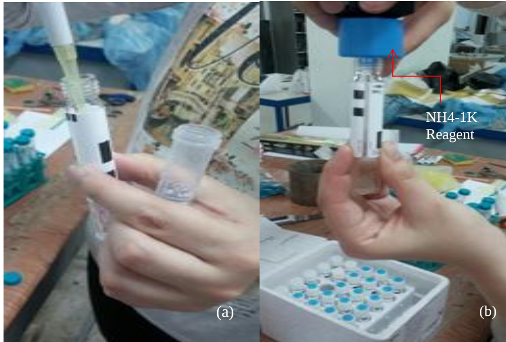
Figure 2.5 Preparation of samples for CEC: (a) Adding 0.1 ml KCl extract and (b) one dose of reagent in a reaction cell (Personal archive, 2016)
