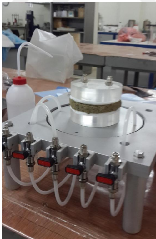
Figure 3 Applying bentonite paste to specimen (Personal archive, 2015)
