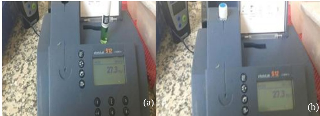
Figure 2.6 Spectrophotometry measurement on colored extract: a) before and b) after analyzing (Personal archive, 2016)
