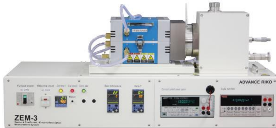
Figure 4.6: Electrical resistivity and Seebeck coefficient measurement system.
