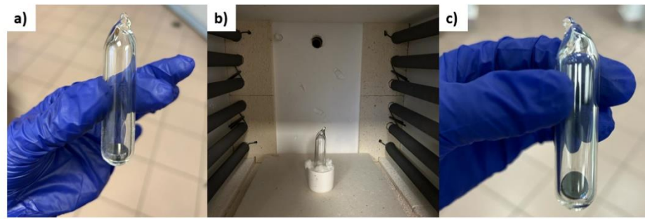
Figure 5.1: a) The material placed in the thin quartz/glass tube, b) The image of the alumina crucible in the furnace, c) The image of the material after annealing.
