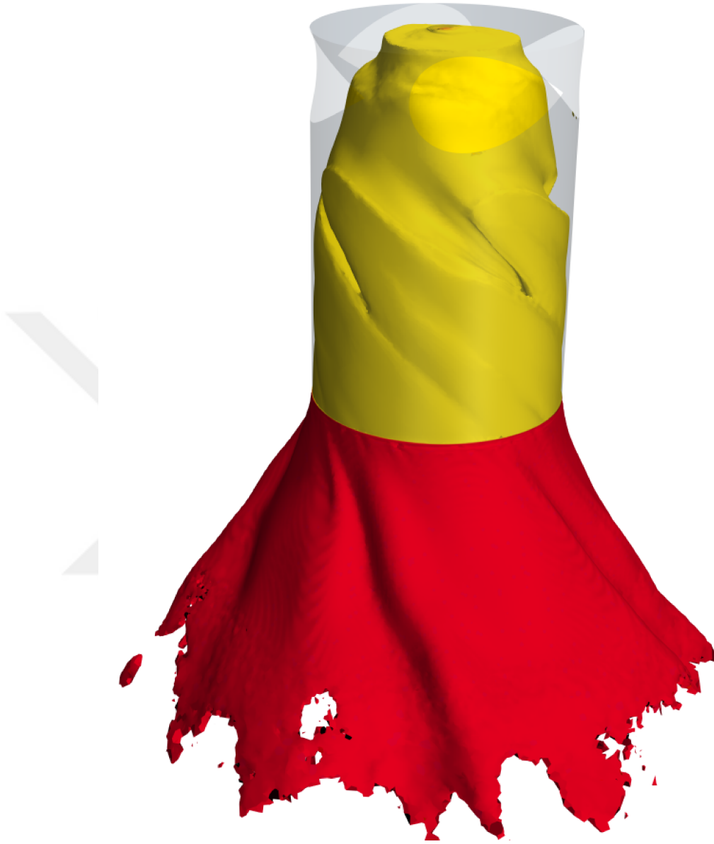
Figure 117: Structure of air core and liquid sheet for Case-13
