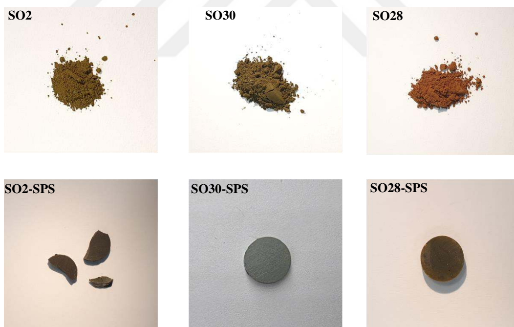
Figure 3. 12 Images of the unpurified powder ZnSe samples synthesized with ball milling method and their corresponding pellets obtained afterwards via SPS.
