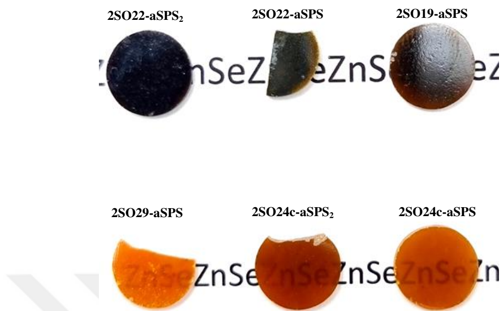
Figure 3. 20 Solid state ZnSe materials synthesized via solid state and sintered to form pellets by SPS.
