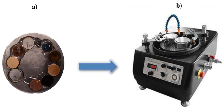
Figure 2. 5 a) The sintered ZnSe pellets prepared for polishing and thickness tuning to 1 mm, b) The polishing device used in thesis work.
