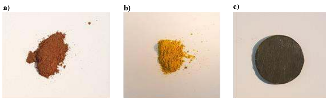
Figure 3. 17 SO11 sample a) after drying in tube furnace (SO11-ad), b) after annealing in tube furnace (SO11-ac), c) after sintering (b) with SPS (SO11-aSPS).
