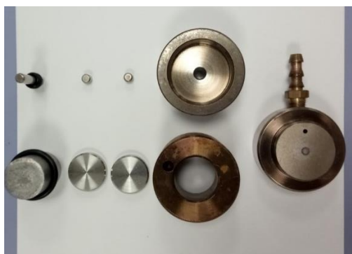
Figure 3.18: Illustration of the Special Mould used for Sample Preparation of the polymeric membranes.
