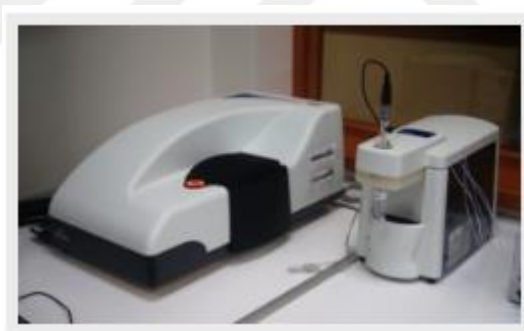
Figure 3.15: Equipment for measuring the hydrodynamic radius of polymers used in this work (DLS).
