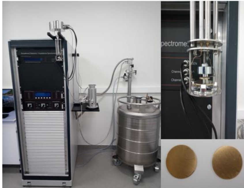
Figure 3.6: The Alpha A analyzer (Novocontrol Co.) equipment for Broadband Dielectric Spectroscopy.
