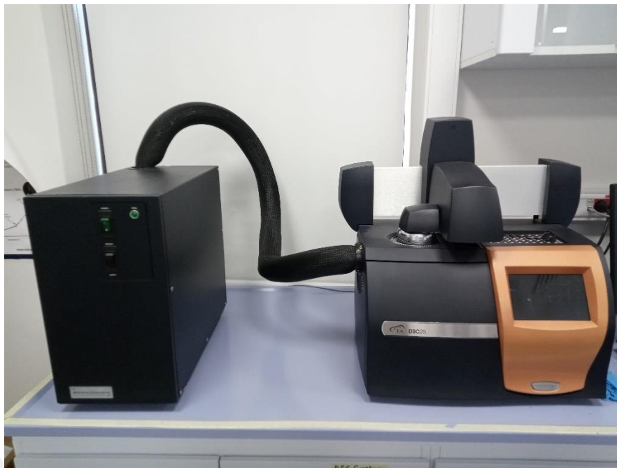
Figure 3.4: TA Instruments DSC25 instrument equipped with a liquid nitrogen cooling system.
