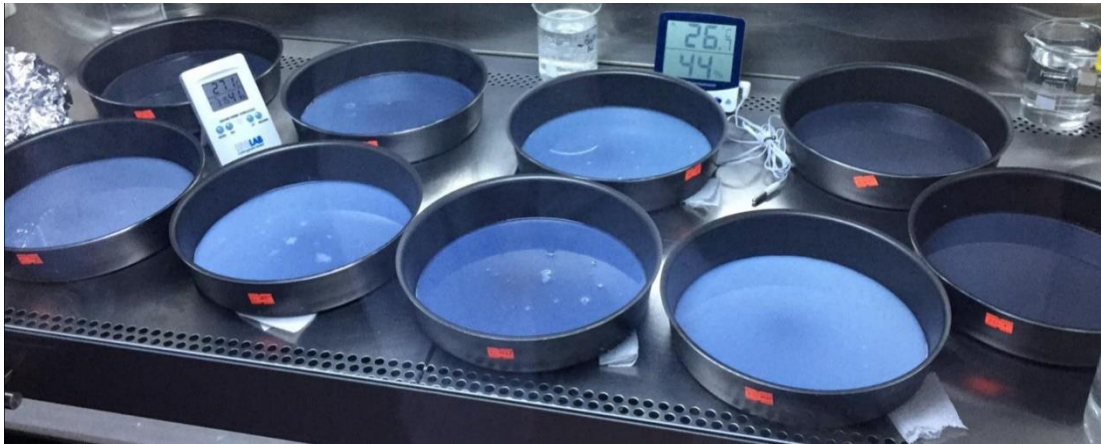
Figure 3.1. WPC film after drying at 25°C, 50%±5 RH for 72 hours
