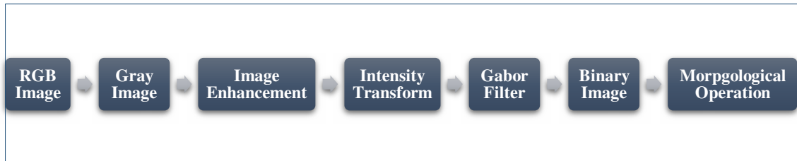
Figure 4.1 Flow chart of the Gabor filter algorithm
