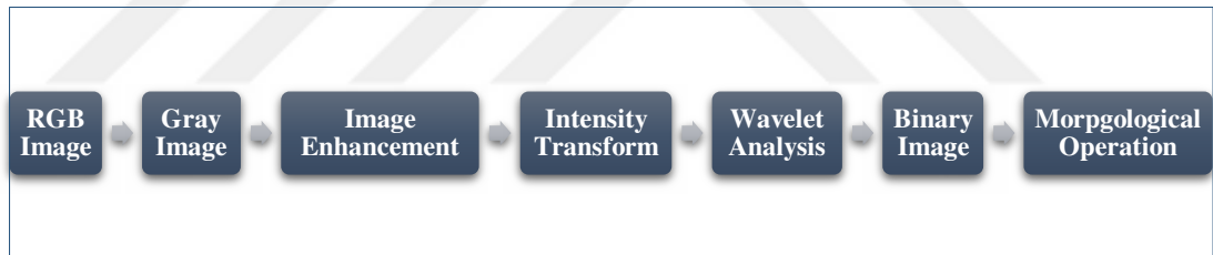
Figure 4.3 Flow chart of the Wavelet filter algorithm
