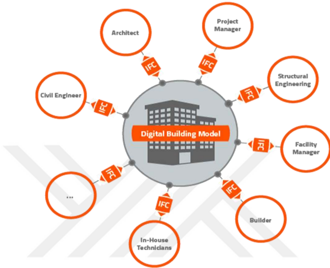
Figure 31: BIM Information Exchange Management
