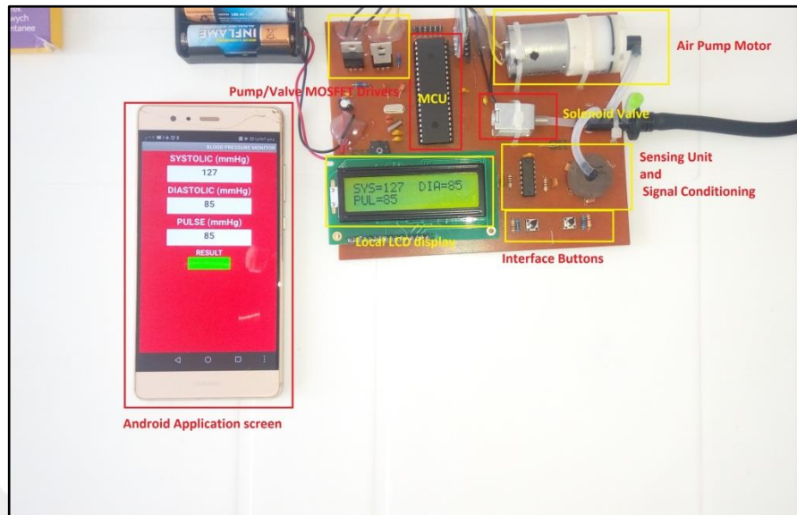
Figure 5.8 System test readings with elements description.
