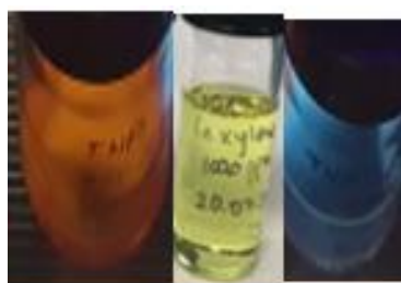
Figure 3.6: Color change under UV light for: TNP, TNP-Melamine, TNP-b-PEI in xylene.
