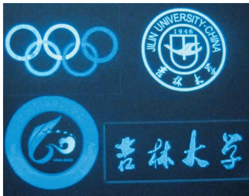
Figure 2.1: Figures created by blue emitting CD based ink (Zhu et al., 2013).
