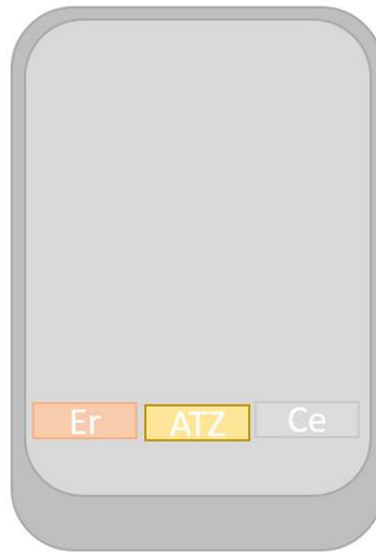
Figure 3.105. Schematic representation of samples in a graphite crucible sintered at 1800 °C.
