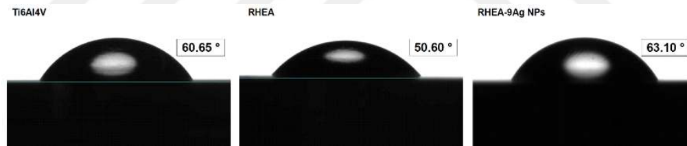
Figure 5. 9. Photographs of a PBS drops and their contact angles measured on the surface of Ti6Al4V, RHEA, and RHEA-9 Ag NPs.
