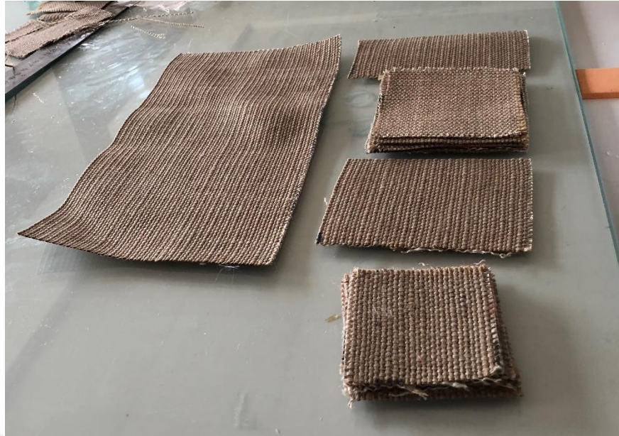
Figure 4.3. Flax/jute fabrics cut according to test standards
