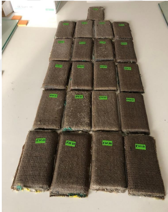
Figure 4.23. Impact test samples
