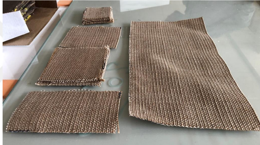
Figure 4.1. The cutting pieces of flax/jute fabric
