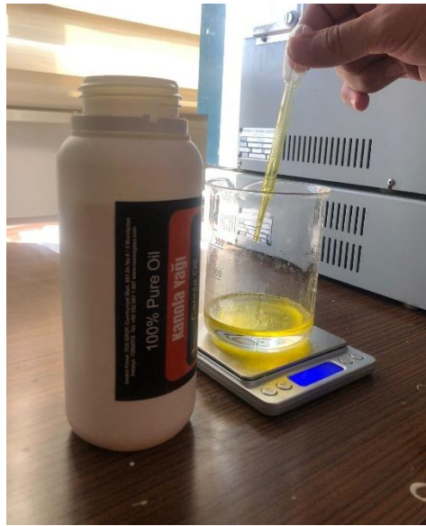
Figure 4.6. Vegetable oil addition to epoxy
