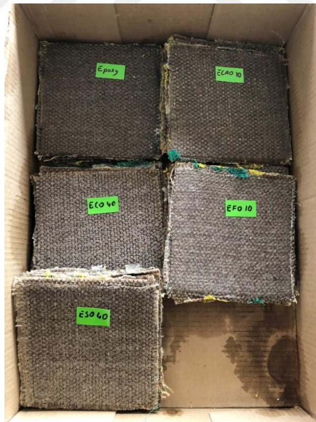
Figure 4.21. Water absorption test samples
