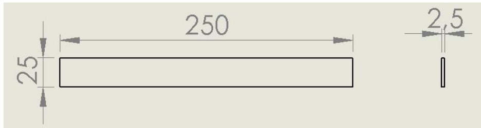
Figure 4.26. Technical drawing of produced tensile test samples (dimensions in mm)
