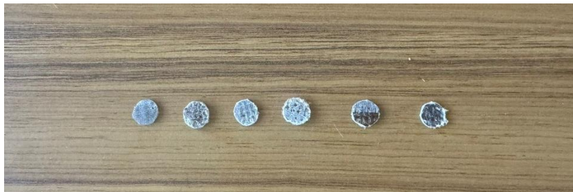
Figure 4.36. Samples prepared for TGA and DSC
