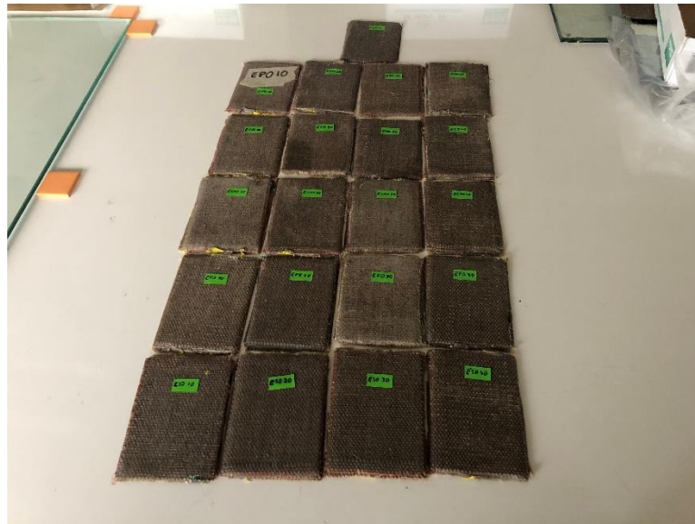
Figure 4.22. Flexural test samples
