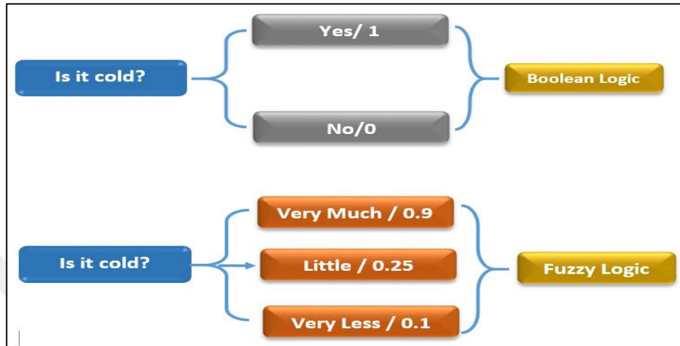
Figure 3.15 Illustrates the differences between Boolean and fuzzy logic.
