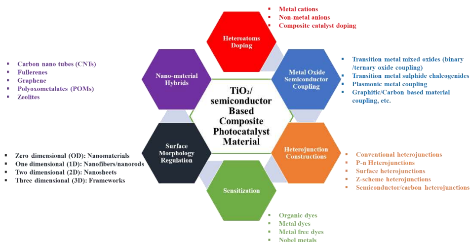
Figure 5. Different modification strategies for the realization of composite photocatalyst material [97, 104, 107]
