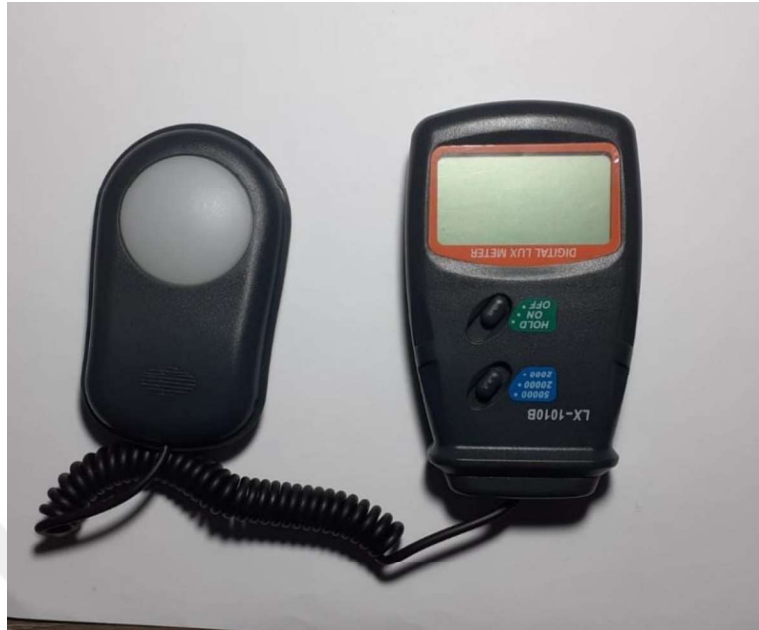
Figure 2.11 Special-purpose lux meter to characterize light sources
