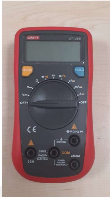
Figure 2.8 Depiction of digital multimeter
