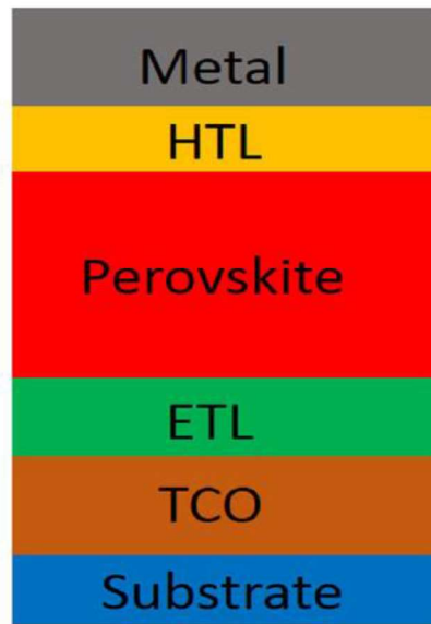
Figure 1.19 Device architecture of conventional perovskite solar cell [32]
