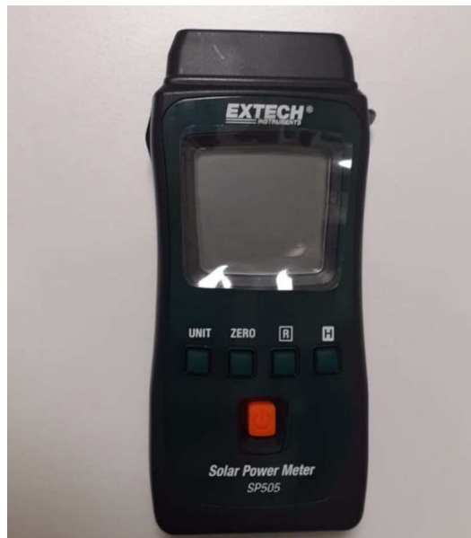
Figure 2.14 Solar power level meter to characterize identical light sources
