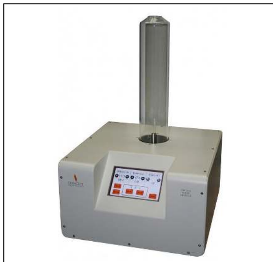
Figure 3.3. The photograph of limiting oxygen index test device
