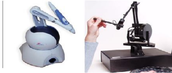
Figure 3 - Sensable Omni and Phantom 6-DOF Haptic Devices
