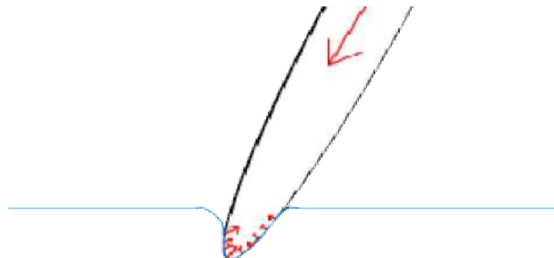
Figure 1 -Reaction forces of a soft-body to the penetrating object
