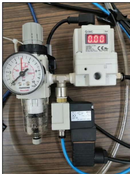
Figure 4.10 Photographic view of the air regulator
