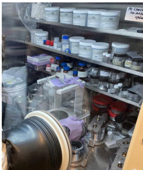
Figure 3.1 Powder loading in the glovebox
