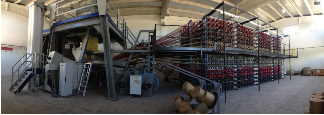
Figure 2.7 Van de Wiele Wilton type face-to-face carpet weaving machine
