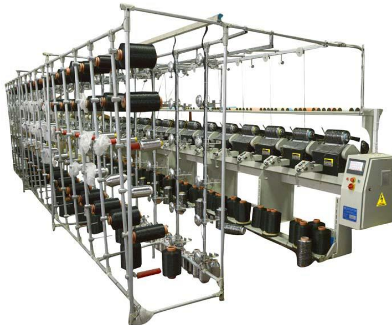
Figure 2.1 AKC-101 plying machine
