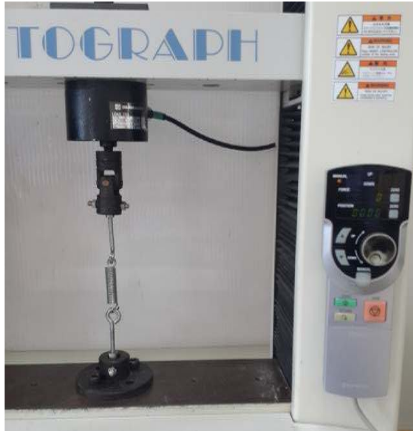
Figure 30. Tension test to determine the k constant value of the spring
