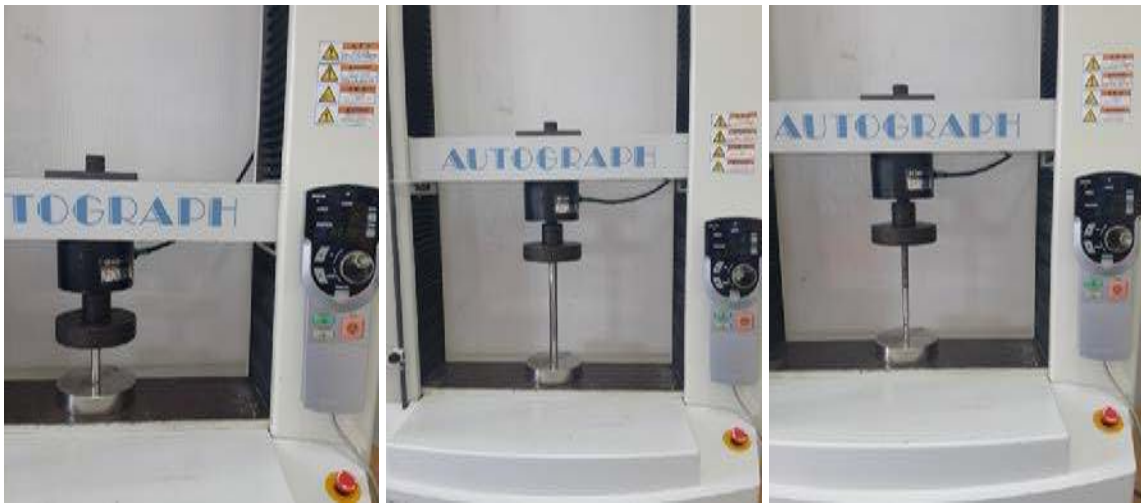
Figure 35. Compression tests of part 1, part 2 and part 3.
