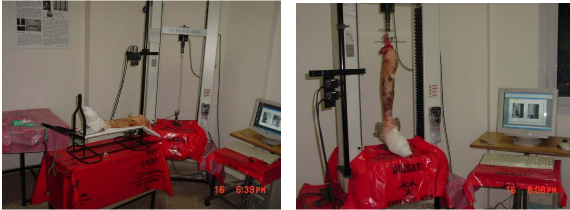
Figure 21. Test set up for measuring the distraction forces.
