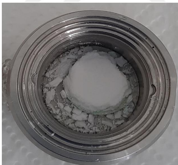
Figure 5.32. Digital image of corroded lithium anode after 48 cycles of the v-Ru/ \alpha\text{MO} electrode.
