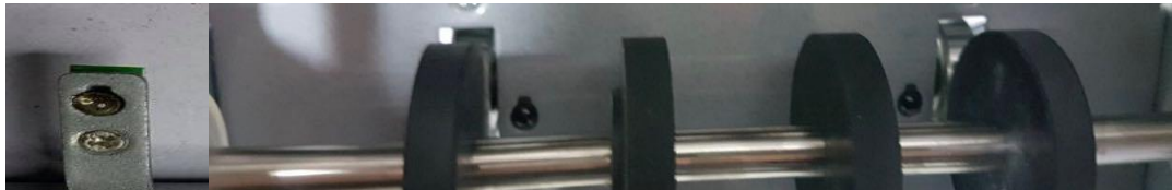
(A)Left, optical transmitter (B) right optical receiver arranged with roller
