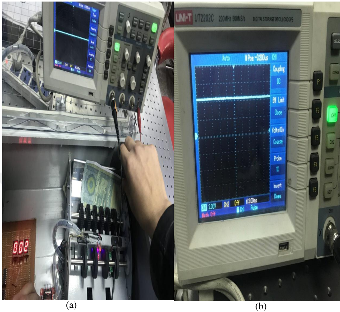
Figure 4.6 the output signal from UV detector when fake 500 Iraqi Dinar (printed currency) passes through the counter
