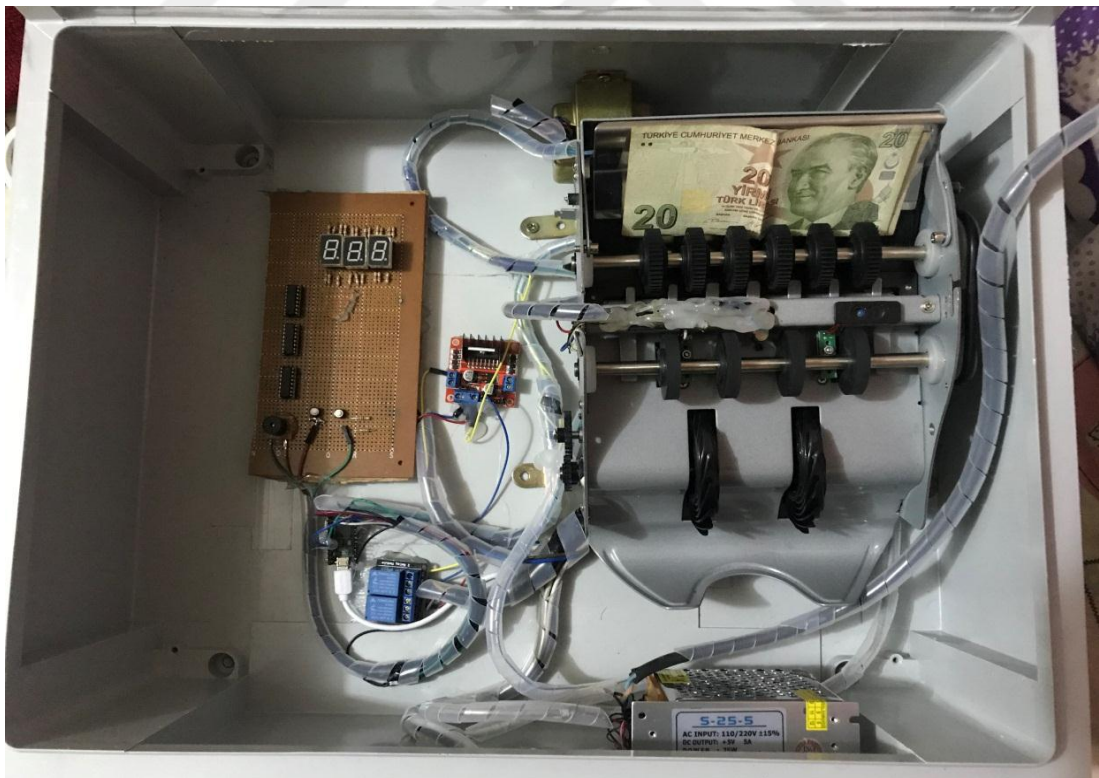
Figure 3.2 Proposed money counting machine (shape, internal structure).
