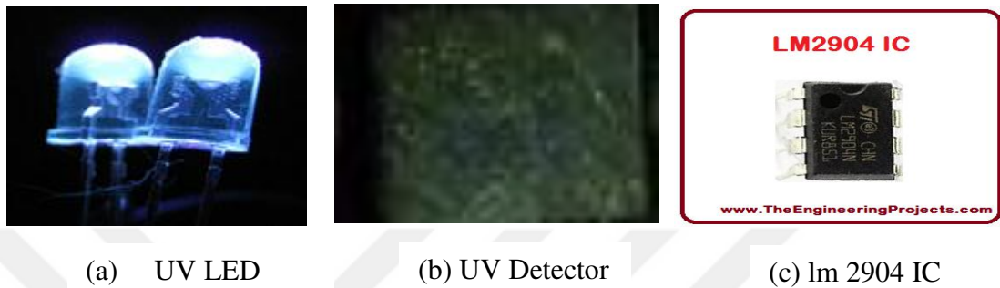
Figure 3.20 UV source and detector system components.
