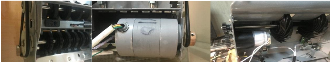
(a) Roller for first stage (b) first stage tying AC motor (c) last stage tying with DC motor
