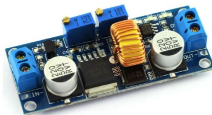
Figure 3.19 The DZS Elec DC-DC step-down constant current regulator used in this study
