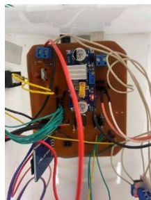
Figure 3.19 The DZS Elec DC-DC step-down constant current regulator used in this study
