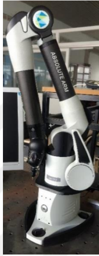
Figure 3.9. Romer absolute arm compact coordinate measurement machine
