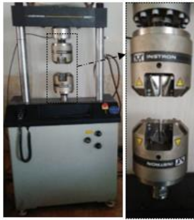
Figure 3.7. Instron 8801 axial fatigue test device
