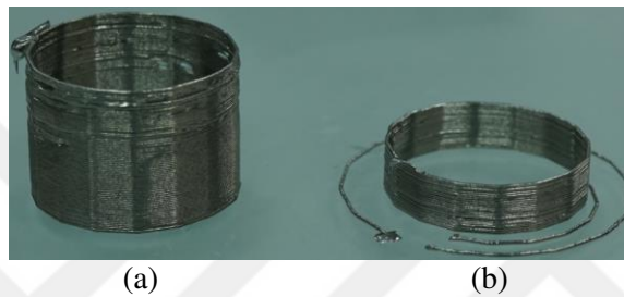
Figure 4.20. Ring samples printed in vase mode
