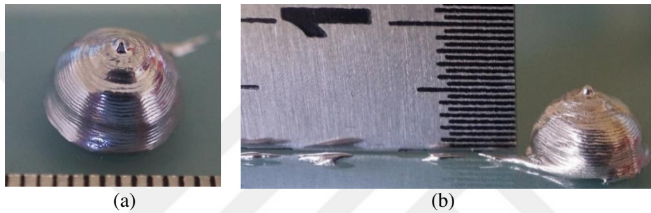
Figure 4.48. Solid hemisphere sample with a diameter of 10 mm printed in start-stop mode using PS of 500 mm/min, LT of 0.2 mm, PT of 75°C, ET of 170 °C, IR of 50%, and EM of 1; a) isometric view and b) side view
