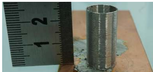
Figure 4.21. The hollow cylinder printed in vase mode
