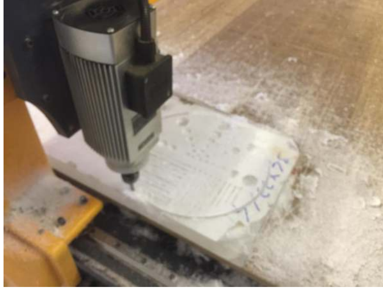
Figure 4.3 A photograph of the in-house phantom under the fabrication process.
