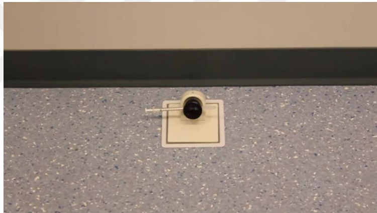
Figure 4.10 A photograph of the point source used for the uniformity test.
