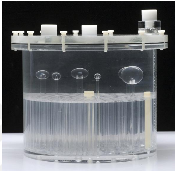
Figure 3.14 Jaszczak phantom employed for checking image quality.
