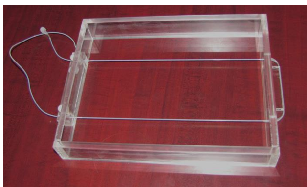
Figure 3.12 Dual-line phantom for whole body resolution tests [102].
