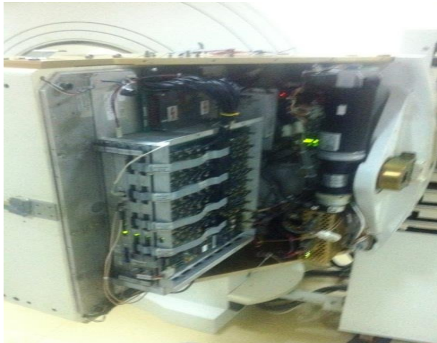
Figure 2.15 \gamma -camera's head electronic systems at GAUN Hospital.
