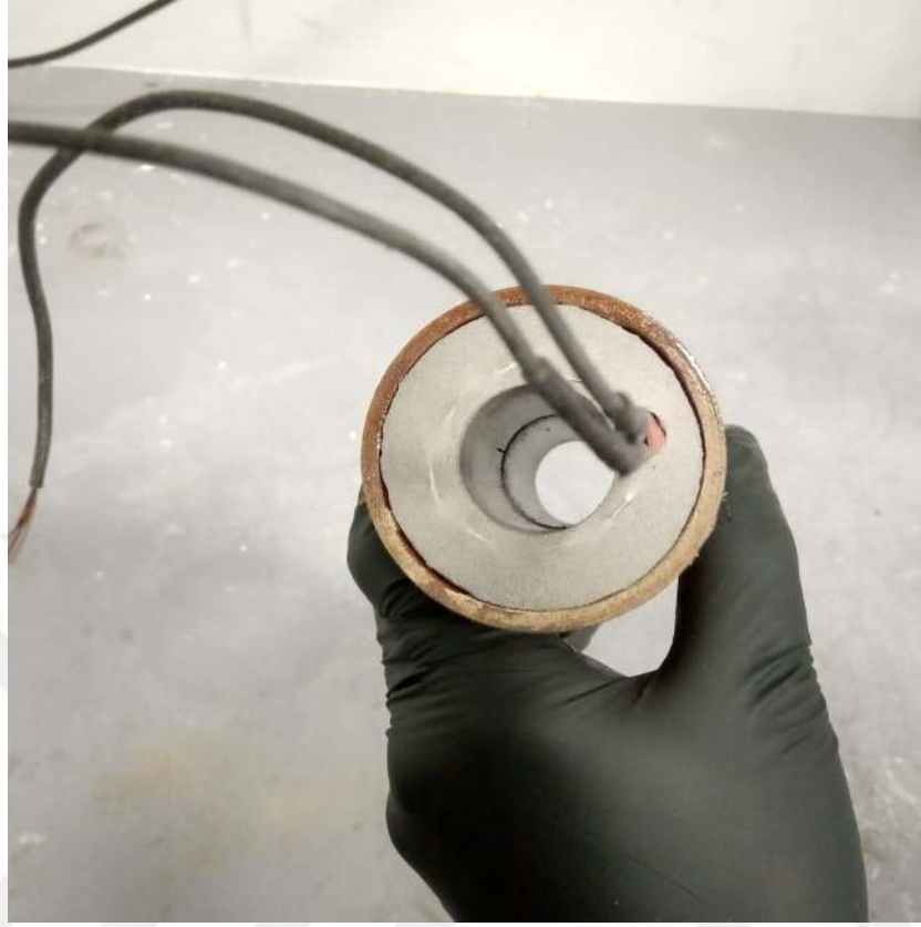
Figure 4.4: Fuel with nichrome wire inserted
