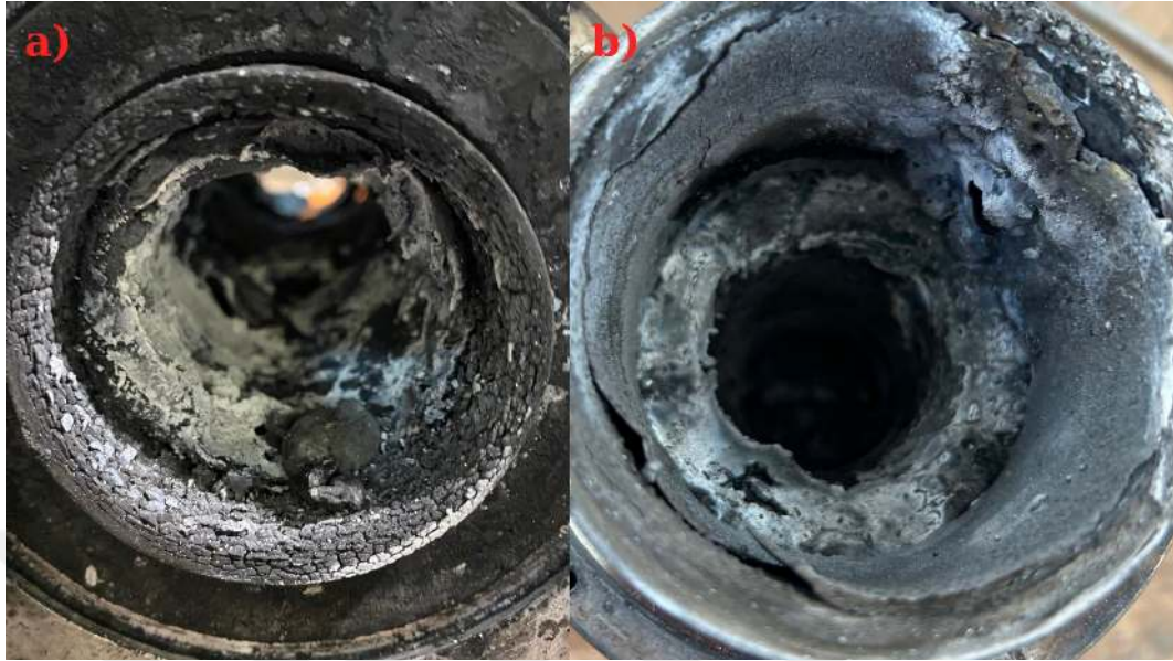
Figure 5.12: Combustion chamber after test of a) Sample 3(5% Binder) b) Sample 6(10% Binder)
