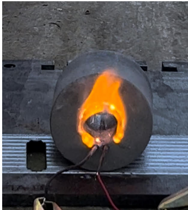
Figure 5.3: Igniter test of 100 bar pressed fuel composition
