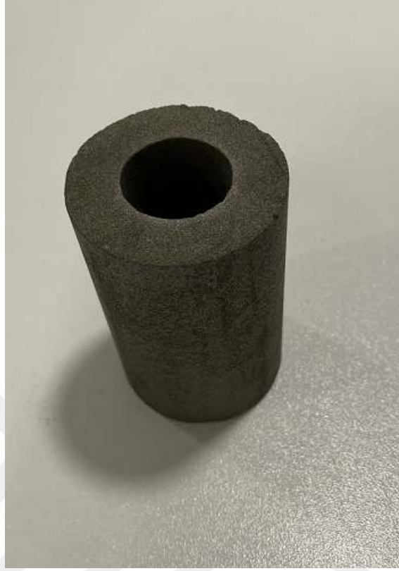
Figure 3.6: Fuel grade (composition: %75 Mg - %20 Al - %5 binder)
