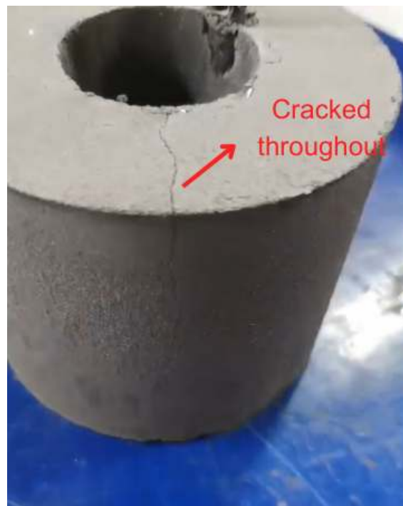
Figure 3.3: Sample subjected to mixing for 1 hour
