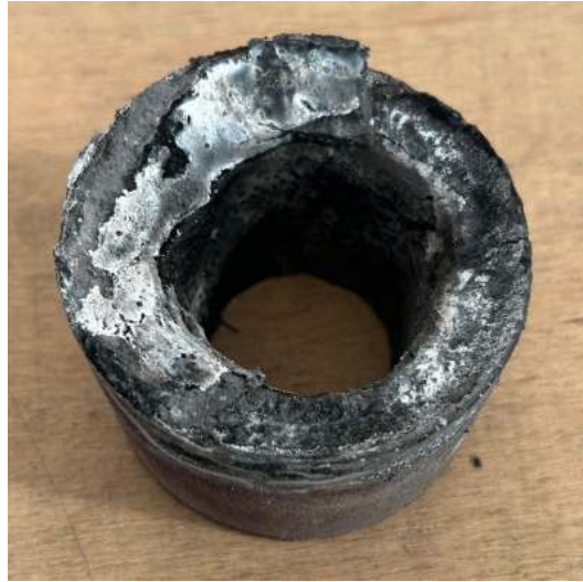
Figure 5.13: Sample 6 fuel Grade after the test
