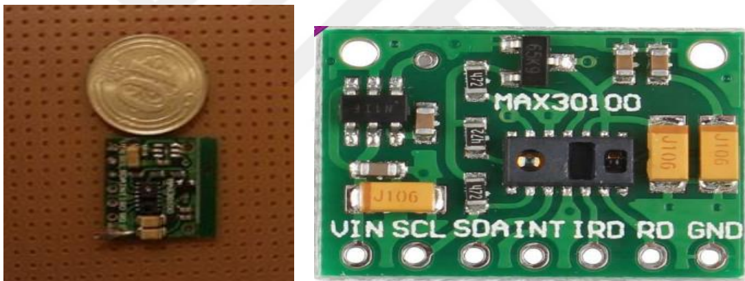
Figure 3.10 The size of max30100 compared with 10 TL coin
