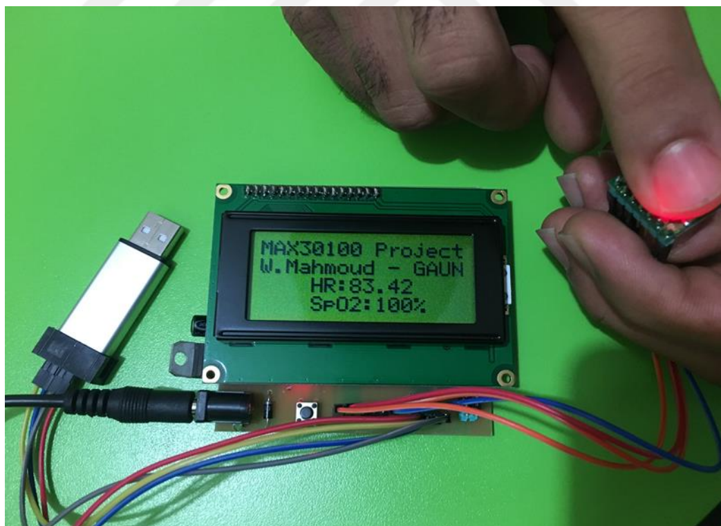
Figure 4.3 the experimental results of the PCB based pulse oximeter
