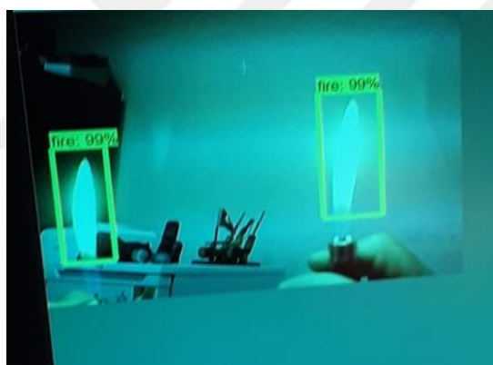
Figure 4.10 Implementation of Fire Detector Software (Personal Archive)
