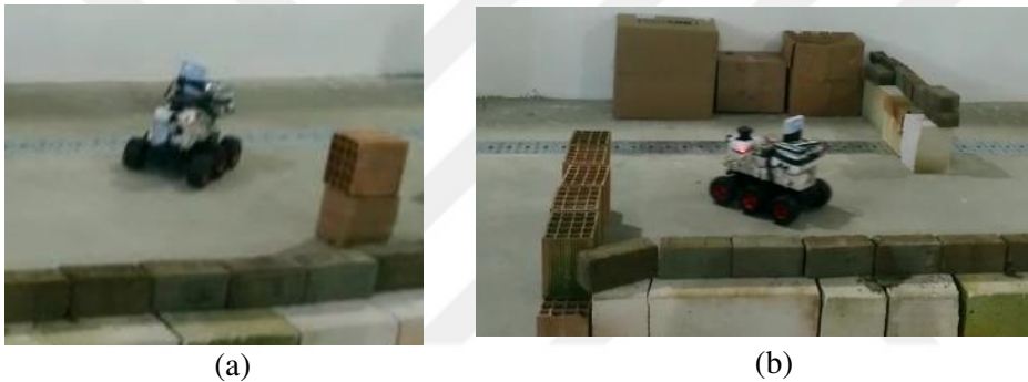
Figure 4.21 Experimental Results from Test Bed Three (a) Front Left Obstacle, (b) Front Right Obstacle (Personal Archive)
