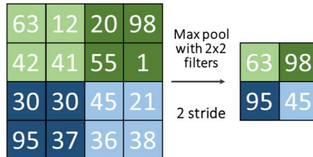
Figure 2.10 Max pooling process and result.
