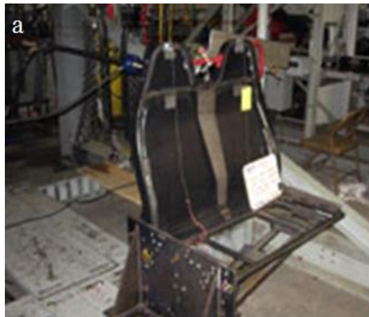
Figure 4.8. Actual APTA Seat Tests Photos a) APTA Horizontal Seatback Load Application b) APTA Vertical Force Application (Anonymous, 2016f)
