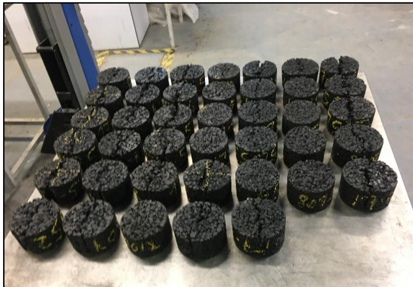
Figure 7.6. Appearance of samples after fatigue test.
