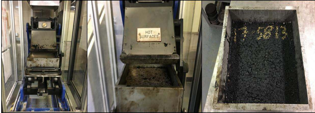
Figure 5.14. Roll press and sample preparation.
