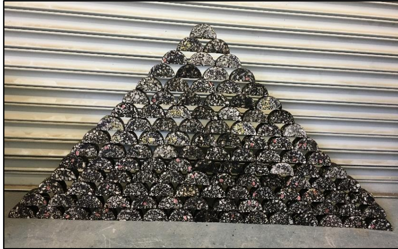
Figure 6.14. 3PB post-test appearance of aged samples.
