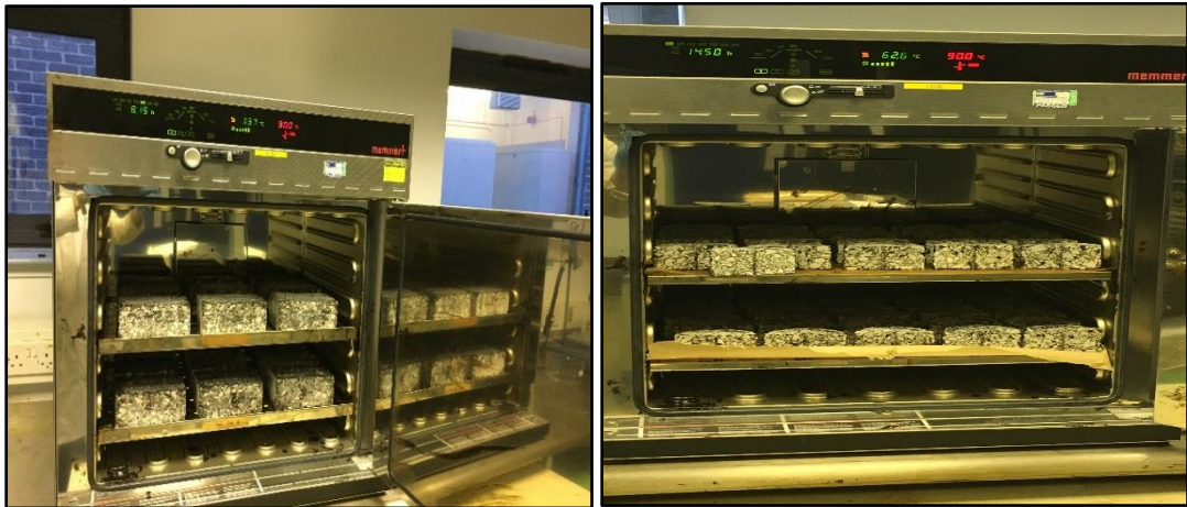
Figure 4.2. Long-term aging of the HMA samples.
