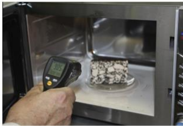
Figure 2.9. Measuring the surface temperature of the specimen [49].
