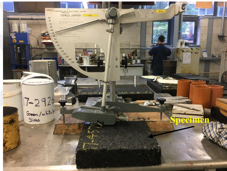
Figure 5.19. Skid test configuration.
