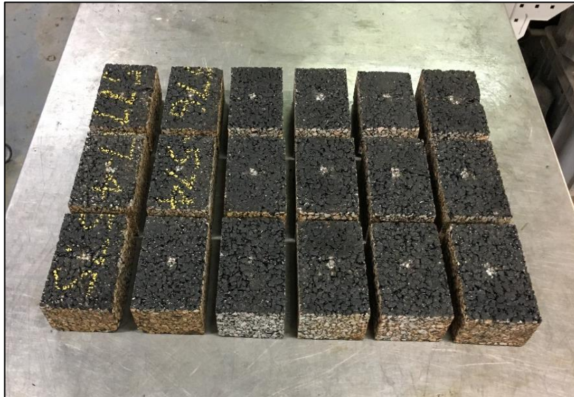
Figure 7.8. Crack healing test samples.
