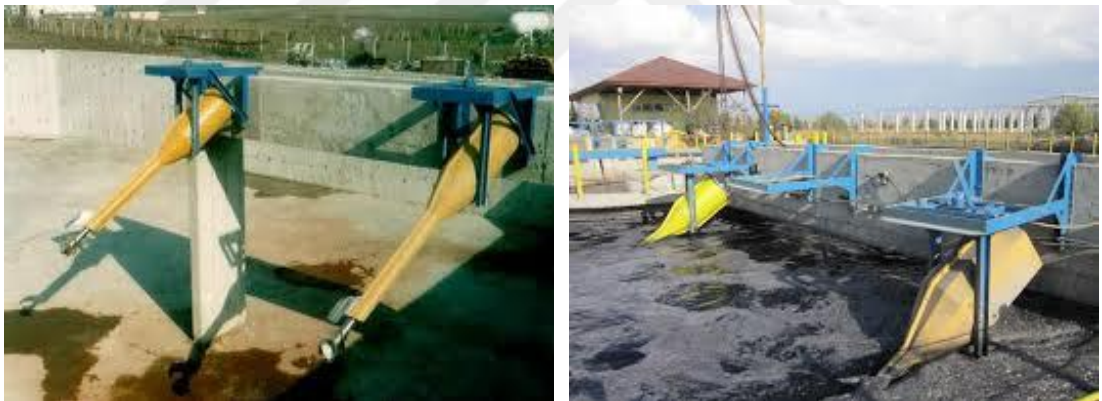
Figure 2.11 Fuchs type aeration
