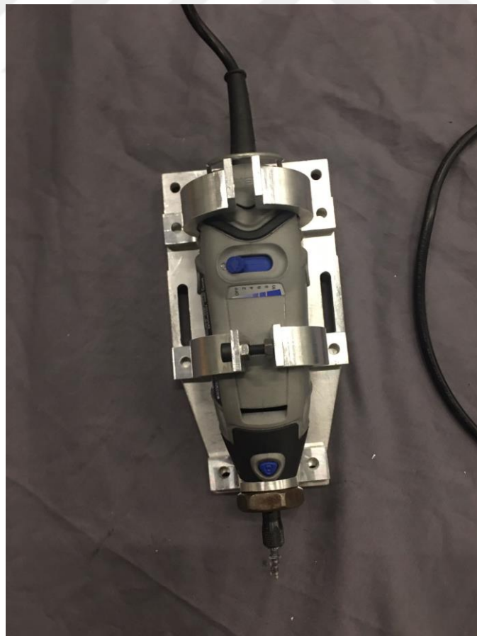
Figure 40: The exemplary assembly of Dremel-EE-2
