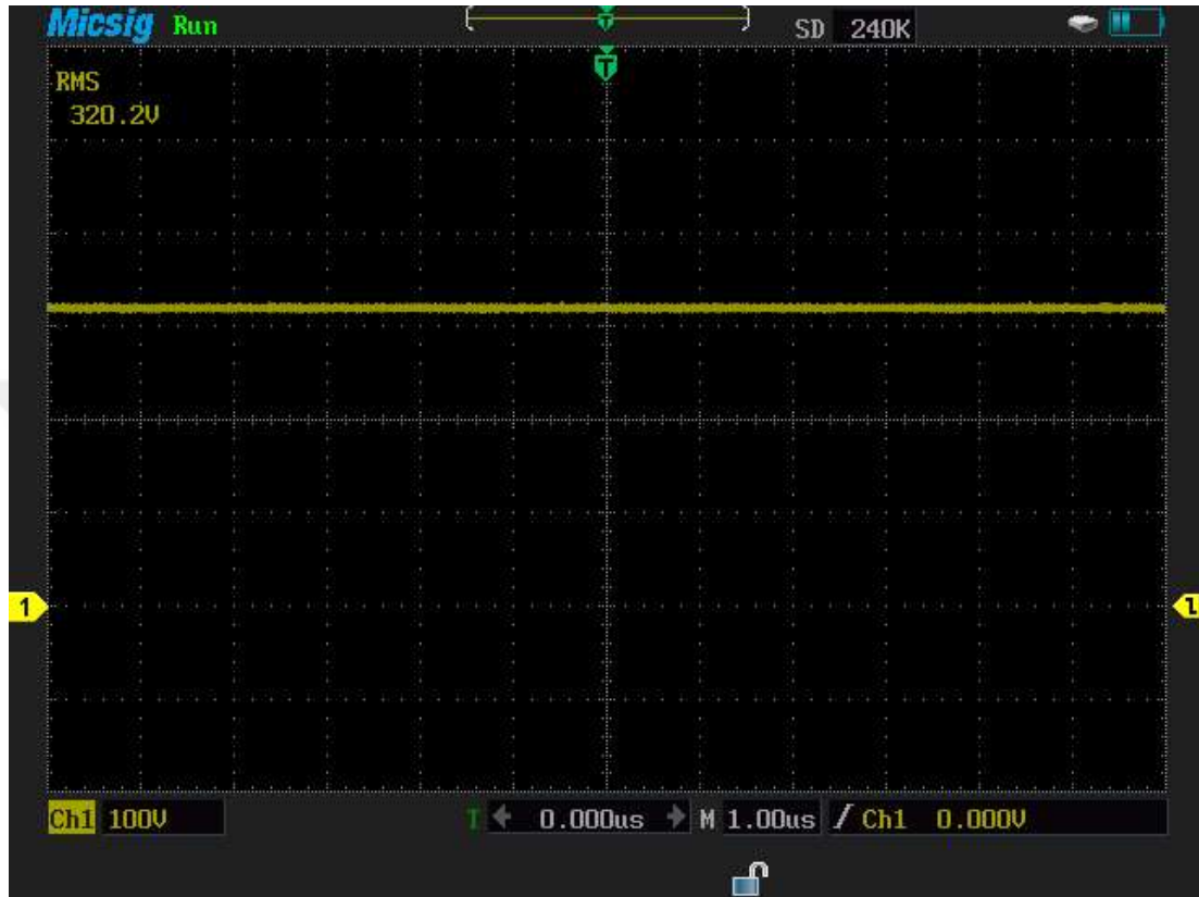
Figure 4.6 Rectified variac voltage
